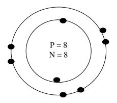
Electrons on the outermost energy level are called <u>valence electrons</u> and determine how the atom will react with other atoms. In the example above, oxygen has 6 valence electrons.
